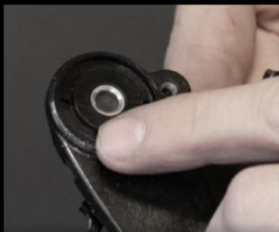
7. There are 2 holes for spring tension. We recommend Low tension setting (marked 'L' at top) to minimize drive train friction. Move the spring tension to the standard setting (at bottom) if you experience any issues such as slow shifting response or drop a chain.
