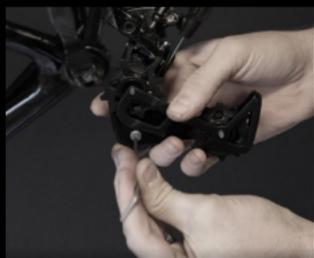
4. Remove the cage mounting screw with a 3mm Allen key and set aside the original cage. You will reuse the cage mounting screw.
