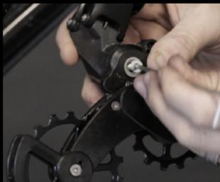
8. Once the spring tension setting is selected, align the OSPW X, spring and derailleur body together. Install the factory cage mounting screw, and torque to 4Nm.
