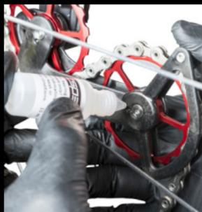
normal conditions, we recommend that you service the Oversized Pulley Wheels when you have ridden under wet conditions, washed your bike or each time you lubricate the chain. For normal maintenance, add a drop of oil into the lubrication points (see the page 3) for optimal performance. Make sure to position the OSPW System horizontally to ensure that the oil reaches the Oversized Pulley Wheel bearings.
