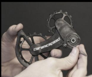
6. Unbox the OSPW X and remove the silver CeramicSpeed stop screw with a 2,5mm Allen key.
