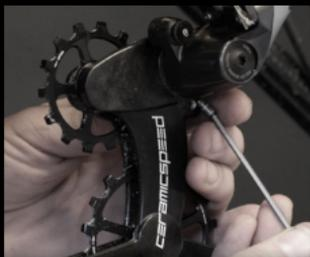
9. Turn the cage clockwise and secure the cage with the Cage Lock. Mount the CeramicSpeed stop screw with a 2,5mm Allen key (torque to 3Nm).
