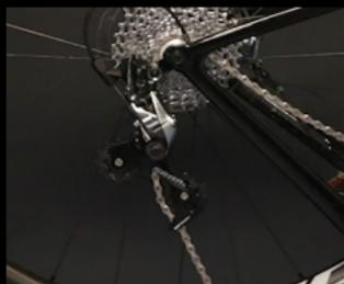
1. Rotate the stock pulley cage forward and engage the Cage Lock. Remove the chain.
