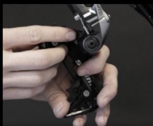
3. Disengage the Cage Lock and release the spring tension to zero. The cage will unwind a complete revolution.
