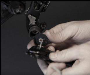
5. Remove the plastic cap if it did not come off with the derailleur cage and set aside (not to be used with OSPW X). You should now see the pulley cage tension spring.
