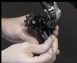
2. Remove the stop screw with a 3mm Allen Key, this will not be reused. Shift up 2-3 gears.
